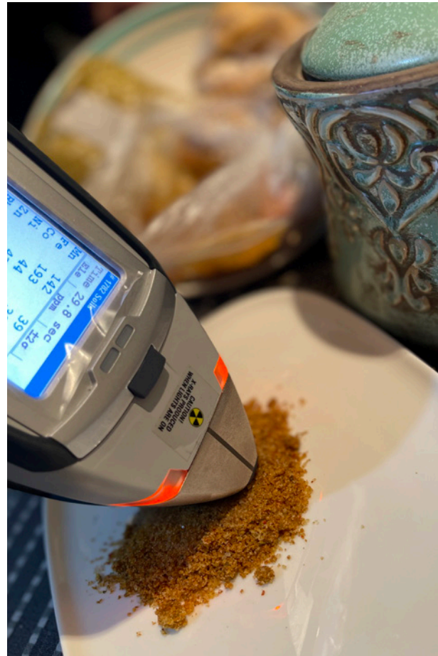
Testing spices for the presence of toxic lead using an XRF (X-Ray Fluorescence) analyzer.
